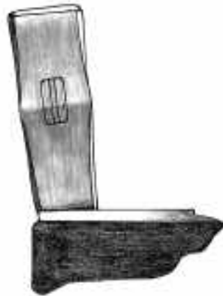
2a. The hammer head is tilted so the peen strikes the bar at the angle of the desired taper.
