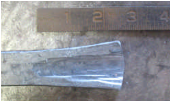
3. Centered trough formed by cross peen, 2 1/2" long.
