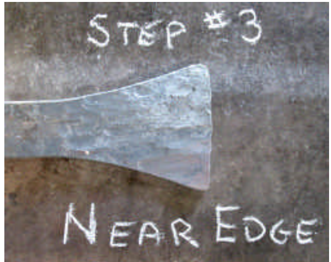
5. Both corners have been peened out in this photo. This is what the fishtail should look like before refining with the face of the hammer.
