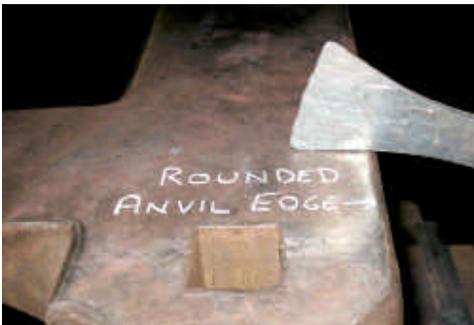
7. This is the position of the fishtail on the anvil to refine the shape. Refine at a low heat to reduce buckling.
