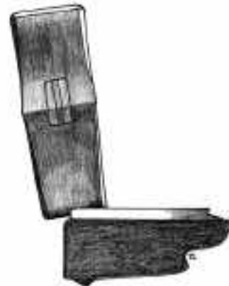
2b. Because the bar is held even with the far edge of the anvil, the corner of the hammer peen should never come in contact with the face of the anvil even if the blow lands a little wide of the mark. Working at a slightly rounded edge will prevent damage to the squarest edge of the anvil, should the bar slip back from the edge.
