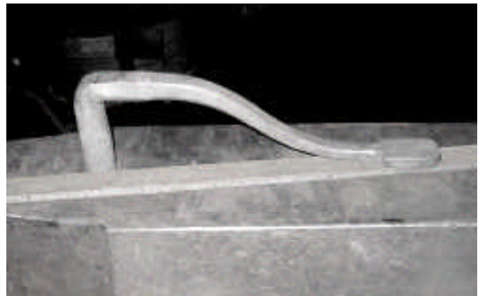
6. The holdfast slides into the pritchel hole, and holds the workpiece firmly with a light tap of the hammer above the holdfast's vertical shank. To remove the holdfast, lightly tap the side of tool's vertical shank with the hammer.
