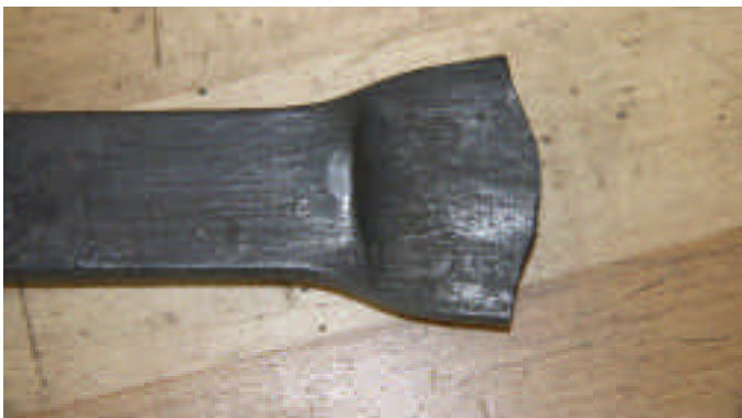
Fig. 11. Bottom of bar showing transition made by rounded corner of the anvil.
