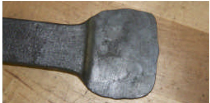
Fig. 17. Flattened bar using the face of the hammer.
