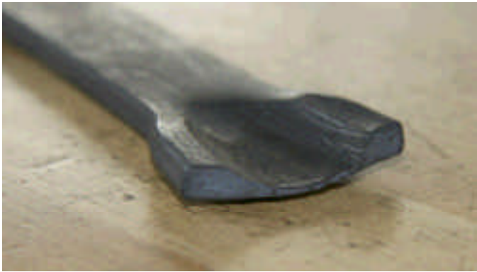
Fig. 10. Top of the bar showing peened middle trough.
