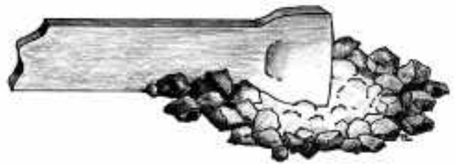
Fig. 13. Half to be worked placed edge down in the fire.
