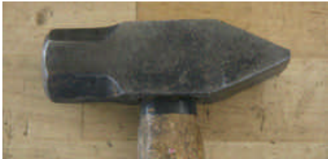
Fig.1 Sharp peen on hammer as purchased.
