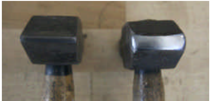
Figs.2 and 3. Reshaped peen ground wider with rounded corners.
