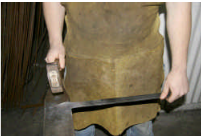
Fig. 7. Stand with shoulder of hammer hand facing the anvil.
