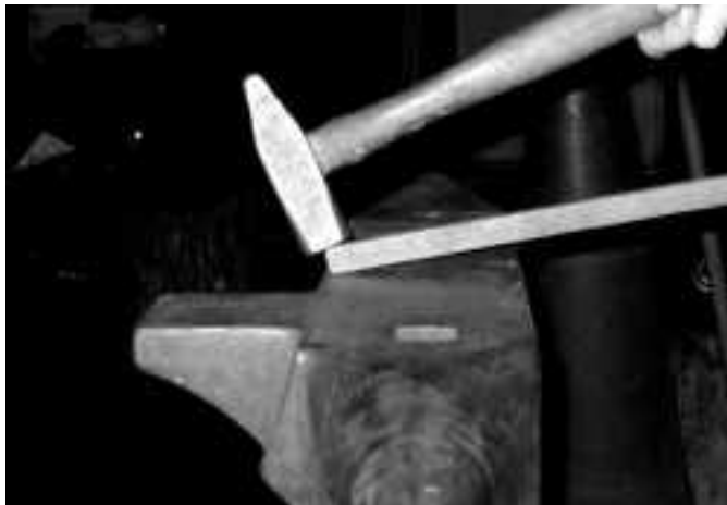
2. Notice the angle of the hammer and of the bar, as well as bar placement on the anvil.
