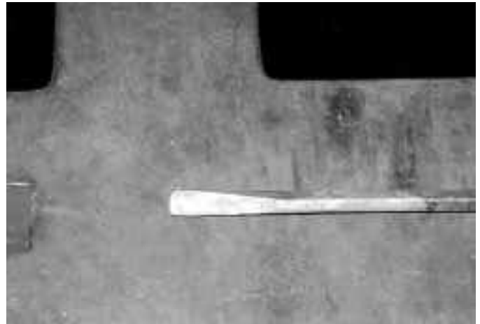
3. Side view of the set-up shape. Notice how the thickness of the parent stock has increased towards the tip.
