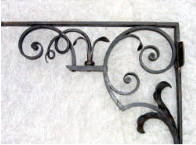
1. Shelf bracket made by Peter Ross. The snub end scrolls were made by making a very long ribbon taper, then tightly rolling the taper to form the snub end. This method of forging snub end scrolls was typical of English 18th century ironwork.
