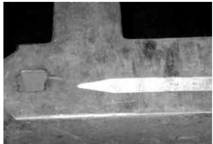
3a. Top view of the set-up shape. Notice that the width of the parent stock has decreased towards the tip.
