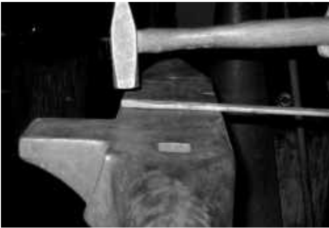
4. Correct position of the bar and set-up shape on the anvil to begin drawing out the ribbon taper.
