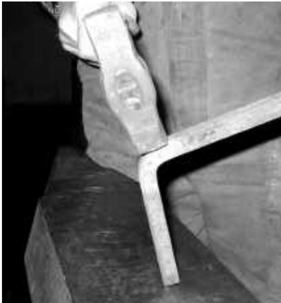
4. Vertical blow- note the position of the hammer and the short leg.
