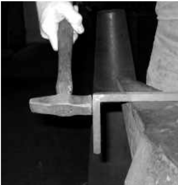
7. When trueing the angle to 90 degrees, keep the short leg away from the anvil as shown here. Doing so will keep you from reducing the cross-section of the bar beneath the parent stock size.
