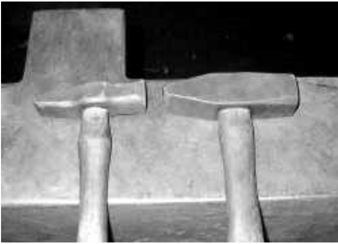
6. Use a smaller hammer to do this operation. The hammer on the left is a one-pound hammer— a good hammer weight for the task. The hammer on the right is a 1.8 pound hammer which is too heavy for this form.
