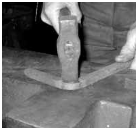
2. Position the hammer as shown when cross-peening the corner. Be mindful that you do not reduce the cross-section smaller than that of the parent stock.
