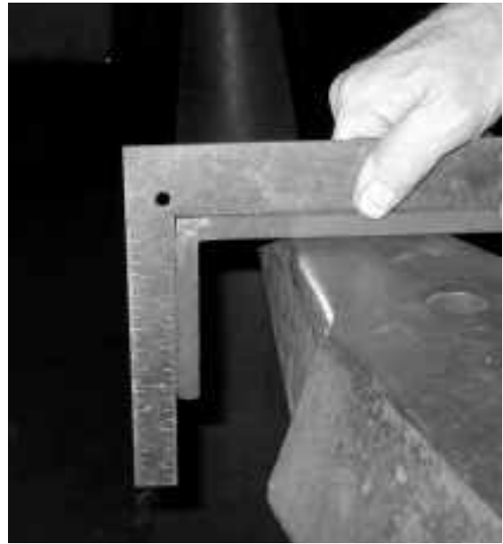
8. Check your work with a square. Note that the legs are square, but there is a gap near the corner of the long leg, which should be corrected.
